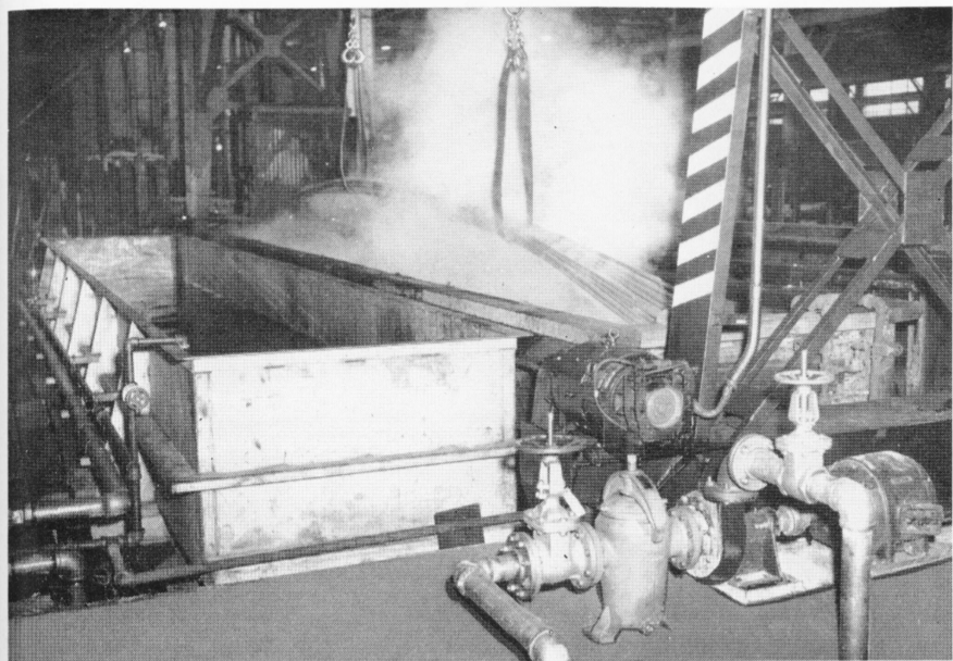
This new stainless steel welded tub is a recent addition in the Tube Mill. In the tank to the right may be seen tubes which are being taken out of their hot water rinse after the bicromate dip and cold water rinse.
